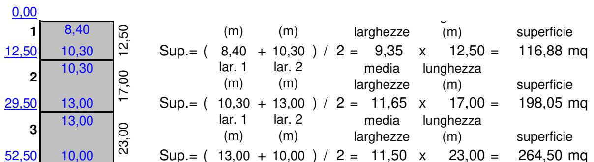
$$\begin{aligned} \text{Sup.} &= (8,40 + 10,30) / 2 = 9,35 \times 12,50 = 116,88 \text{ mq} \\ \text{Sup.} &= (10,30 + 13,00) / 2 = 11,65 \times 17,00 = 198,05 \text{ mq} \\ \text{Sup.} &= (13,00 + 10,00) / 2 = 11,50 \times 23,00 = 264,50 \text{ mq} \end{aligned}$$
